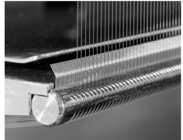
60  $\mu\text{m}$  wires part of the SPS electrostatic septa
